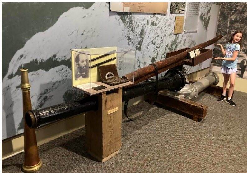
Water cannons were used to wash the gold out of the hills in northern Georgia
